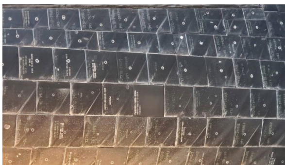
Figure 3. The heat shield tiles on the Space Shuttle show the stretch marks (credit: Hyunju Lee, Smithsonian Science Education Center)
