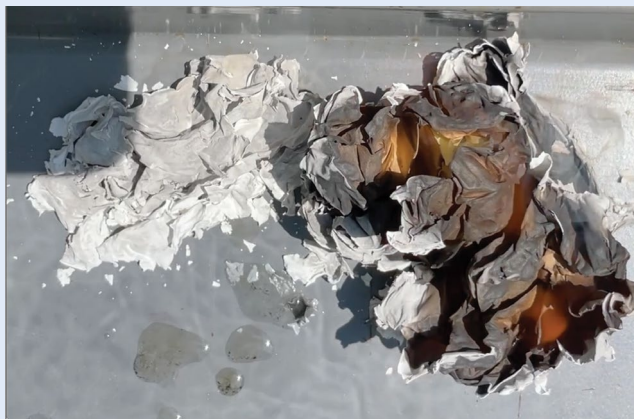
Figure 3.7: Biofuel A (left) has completely burned and turned to ash. Biofuel B (right) is still burning.
