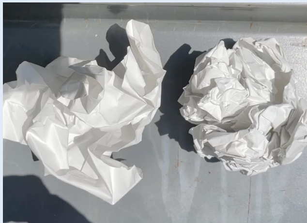
Figure 3.5: Example of Biofuel A (left) and Biofuel B (right); Biofuel B is made out of several sheets of crumpled paper that have been compressed together.
