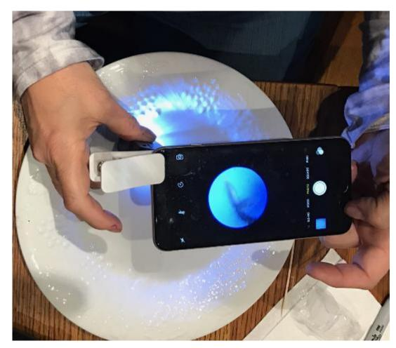
Note that many clip-on devices have a clear collar on them at the end of the lens. You can rest the collar of the lens on your plate.
