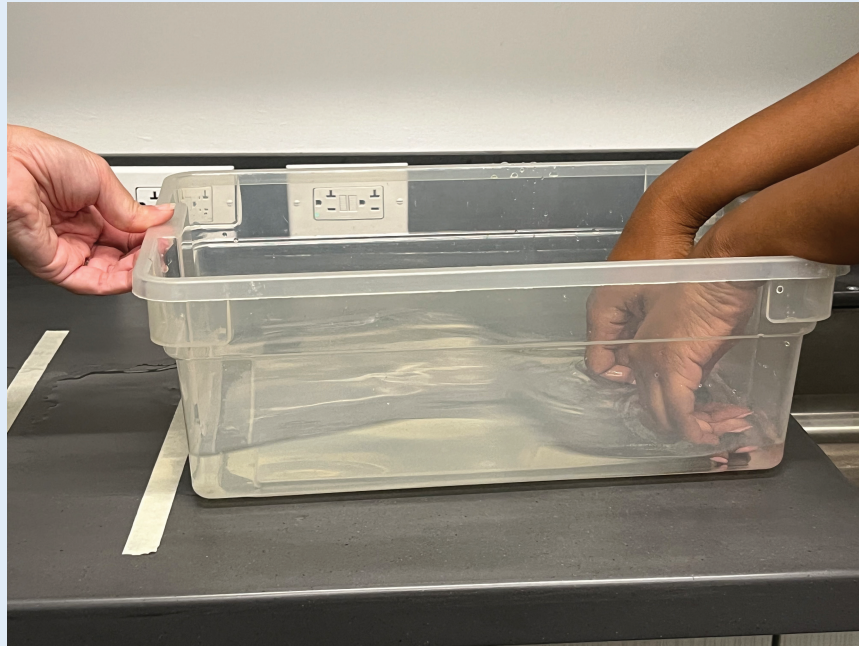
Figure 6.6: One partner pushes the container from the back to the front line to create a wave that washes over the other partner's fingers.
