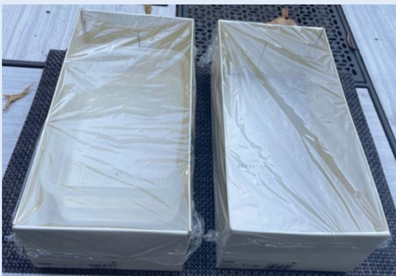
Figure 4.2: Heat sink model setup; the box on the left has a container with water, the box on the right does not.
