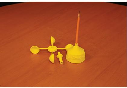
Teacher Tip: Putting a 1-inch metal washer between the spinner piece and the anemometer cups can reduce friction, allowing for more rotations.
