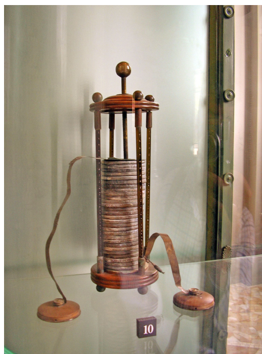
Above: Alessandro Volta's voltaic pile (battery) on display in the Tempio Voltiano (the Volta Temple) near Alessandro Volta's home in Como, Italy Right: A diagram of the voltaic pile (Source:
